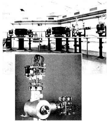
Injection Beamline with Beam Diagnostic System for the Cooler Synchrotron COSY (Forschungszentrum Jülich)
