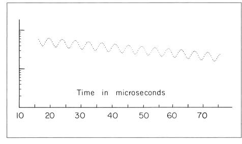
trajectory, which takes about 4 microseconds. It is this modulation period which must be measured very precisely, to 1.3 picosecond.
